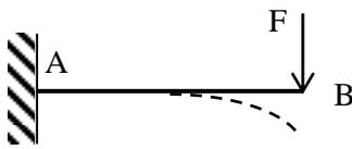
$$\begin{aligned} \theta_A &= 0 \\ y_A &= 0 \\ M_B &= 0 \end{aligned}$$
